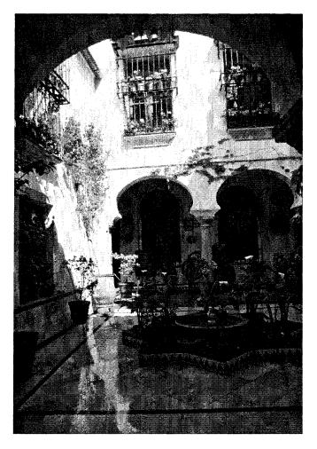
Fig. 2. Polished marble floors are very durable, connote wealth, and reflect light, but such non-porous surfaces do little to aid evaporative cooling. Cordoba, Spain, Calle Encarnacion. From John S. Reynolds, Courtyards: Aesthetic, Social, and Thermal Delight (New York: John Wiley and Sons, 2002; page 36.)
